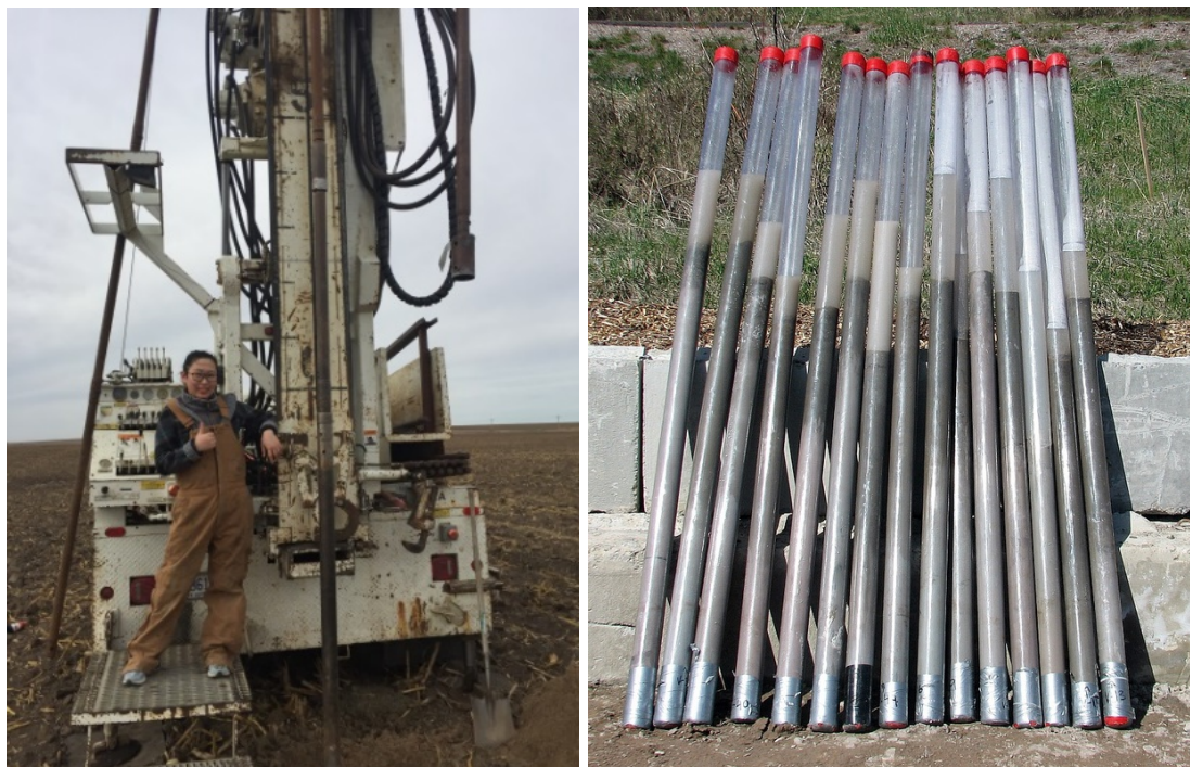
Figure 1. Set-up of drill rig (L) and soil cores prepared for transport to Water Sciences Laboratory (R)
